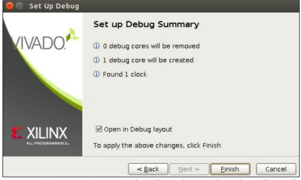
After the setup is finished, go to the left panel and click **Project Manager->Program and Debug->Generate Bitstream**. This will ask you if you want to run the implementation first, to what we answer 'Yes'. This will prepare the bitstream with which we are going to program our device and debug our design.
