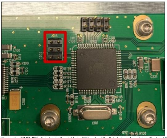
Connect the ATMEL-ICE's 6-pin header (female) to the SPI header of the Octoclock as shown below. The tab of the header must be facing the ATmega128 chip.
