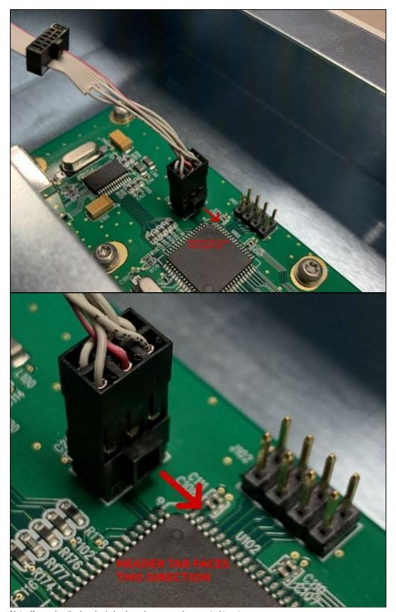
Note: If you plug the header in backwards, avrdude is expected to return a please check your connections message after a programming failure. See the section "Troubleshooting" at the bottom of this document for more detail.
