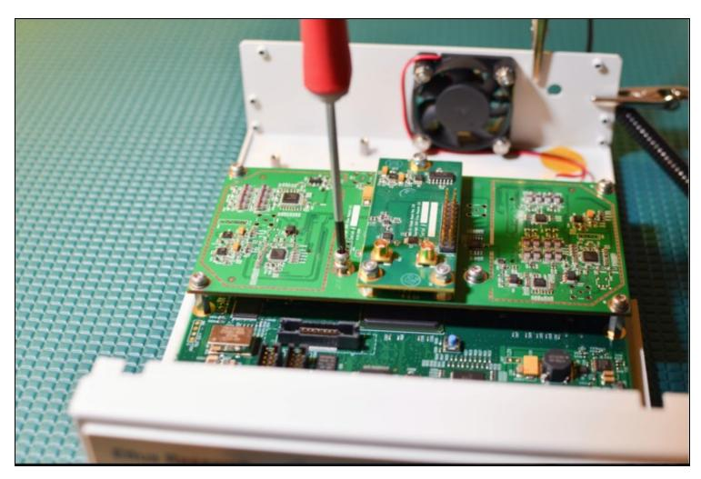
It is recommended to connect the bulkhead cables one at a time to avoid confusion. Note which front panel point (RF1, RF2) you install each connector from the daughterboard to (TX/RX, RX2).
