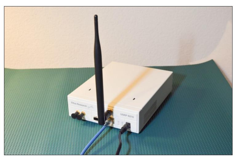
On the computer(host) you plan to use to connect to the USRP set the Ethernet adapter to have an IP address of 192.168.10.1 with a subnet mask of 255.255.255.0. Connect the other end of the Gigabit Ethernet cable to your computer.
