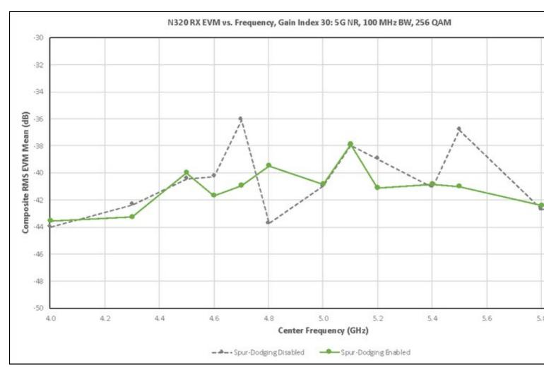
The USRP N320/N321 receiver with the 5G NR modulation standard exhibits excellent EVM performance. This performance can be further improved by taking advantage of the RX I/Q calibration utility available in UHD as well as the spur-dodging algorithm unique to the USRP N320/N321.
