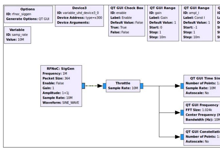
You can see that there is a number of options which can be modified. As we choose to check how signal such as "Wave type" and "gain", we are going to focus on this for now. They can be modified on runtime, but every time that they are set to a different value the trigger has to be run again on the Vivado chipscope. Following are some of the expected results:
