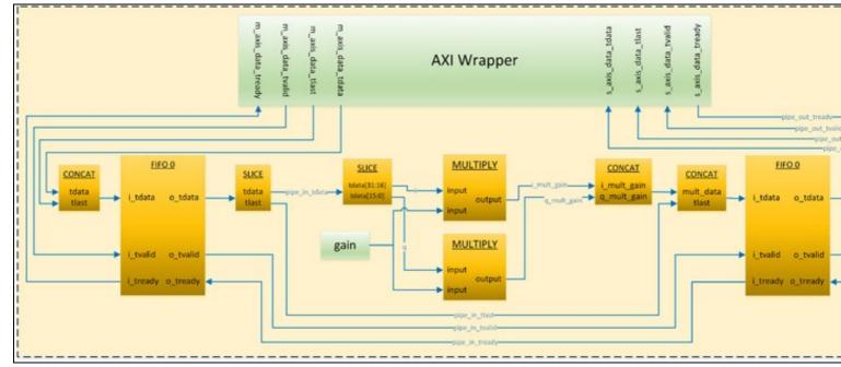
NOTE: In order to meet timing, FIFO blocks were added to either side of the Multiplication process.
