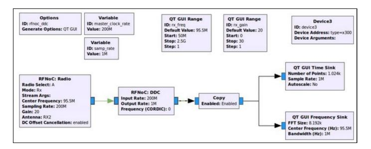
The USRP Source and Sink blocks use the <code>multi\_usrp</code> API, whereas the <code>RFNoC:Radio</code> block uses the RFNoC API. In general, unless RFNoC features are desired, there is no need to use the <code>RFNoC:Radio</code> block. The <code>RFNoC:Radio</code> block is most useful when its output is connected directly to another RFNoC block. Below is a list of differences as well as a GRC screenshot to help differentiate between the two blocks.
