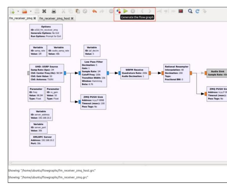
Note: After running the Generate function, within the console of GNU Radio Companion, it will print the location of the generate Python file. The filename will match the value of the ID setting within the Options block.
