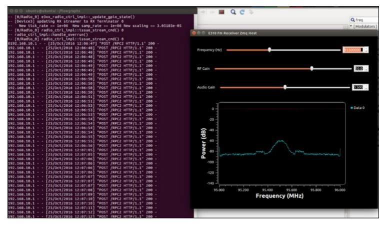
Stopping the application is a multiple step process. First you will need to Kill the flow graph running on the host computer. This can be done by either hitting the "X" in the upper corner of the QT widget window, or by using the "Kill the flow graph" button within GNU Radio Companion.
