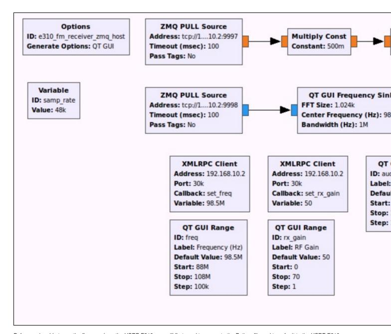
Before you're able to run the flow graph on the USRP E310, you will first need to generate the Python file and transfer it to the USRP E310.
