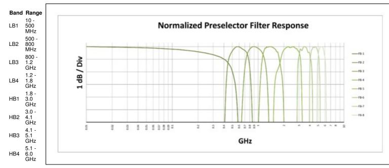
• Each preselector filter has a ±40 MHz band overlap.
