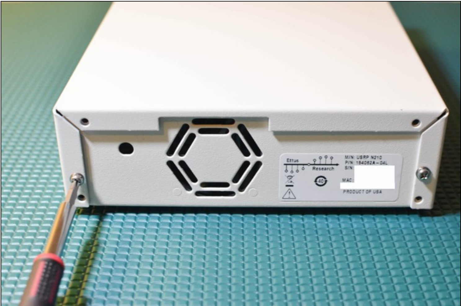
Install USRP cover with screws
