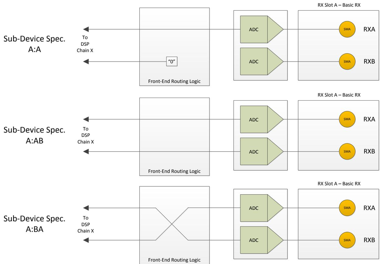
Figure 2 - BasicRX Routing w/ Various Sub-Device Specifications
