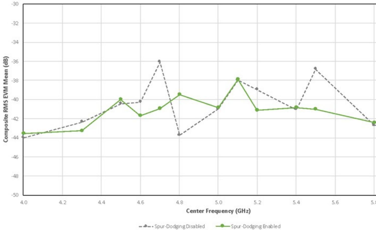
The USRP N320/N321 receiver with the 5G NR modulation standard exhibits excellent EVM performance. This performance can be further improved by taking advantage of the RX I/Q calibration utility available in UHD as well as the spur-dodging algorithm unique to the USRP N320/N321.
