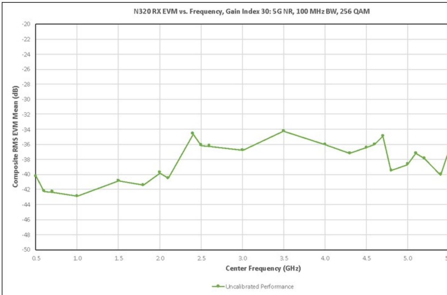
One key contributor to EVM performance is the image level. Images are generated by the I/Q demodulator in the signal chain and are an artifact of this receiver architecture. The image level can be measured and accounted for using the I/Q image calibration utility available in UHD, as shown in the example below.
