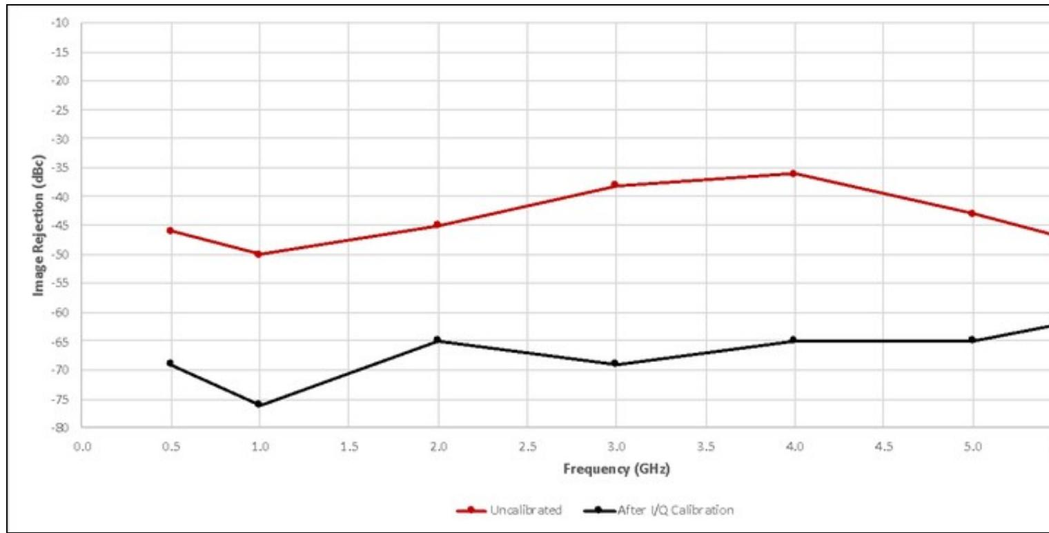
The EVM versus frequency was measured once again after applying the RX I/Q calibration. Significant improvements can be observed as demonstrated in the following comparison plot:
