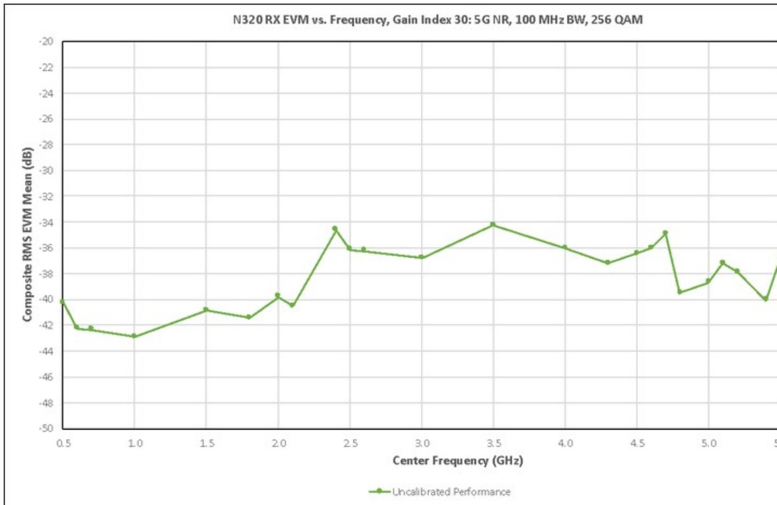
One key contributor to EVM performance is the image level. Images are generated by the I/Q demodulator in the signal chain and are an artifact of this receiver architecture. The image level can be measured and accounted for using the I/Q image calibration utility available in UHD, as shown in the example below.
