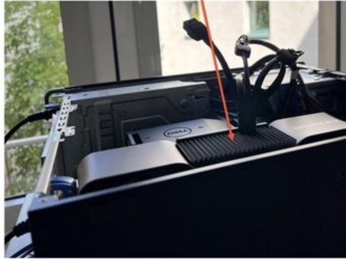
Left: Installed RTX 4090 GPU with ordered power cable. Right: Cover cannot be closed due to cable protrusion.
