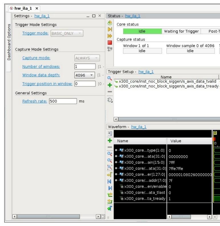
This is what we came for. The block is to be put in a normal use case where it will run and, simultaneously, we will probe signals from it. For the **RFNoC:** Signal Generator, we are going to use GNURadio to set up the application. Actually, we are going to use the siggen example that is shipped within *gr-ettus*. We open to {fpga-repository}{path\_to\_gr-ettus}/examples/rfnoc/rfnoc\_siggen.grc, where a simple setup is ready to show the siggen working.
