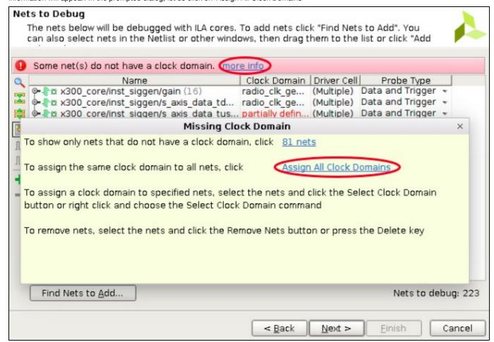
A window will appear where you can choose the common clock domain on which you want to have the signals. Here, in our case, we select radio\_clk\_gen/inst/CLK\_OUT1, and that would be sufficient to continue. Accept and click next.
