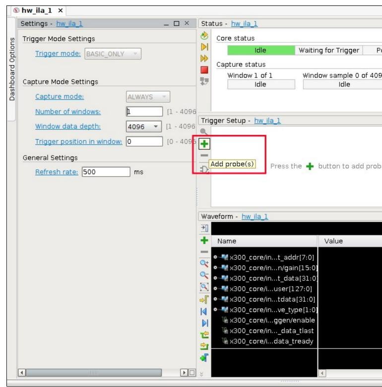
Here we are going to choose two signals as triggers, which are **s\_axis\_data\_tvalid** and **s\_axis\_data\_tready**. The names are almost self explanatory: they state when the device has valid data and when it is ready (see [4] for further information). After choosing this signals, now we have to put our device to work. Even, you can click on "run trigger for this ILA core", which will let the device on idle state waiting for the trigger.
