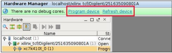
As a first step, click on "Program device". Usually, again, Vivado picks up the bitstream that you just generated. However, if you have been running multiple bitstream builds and/or have multiple Vivado projects, it is possible that you would have to look for the right bitstream. It should be under the project that you have been working during the generation of your debug bitstream.
