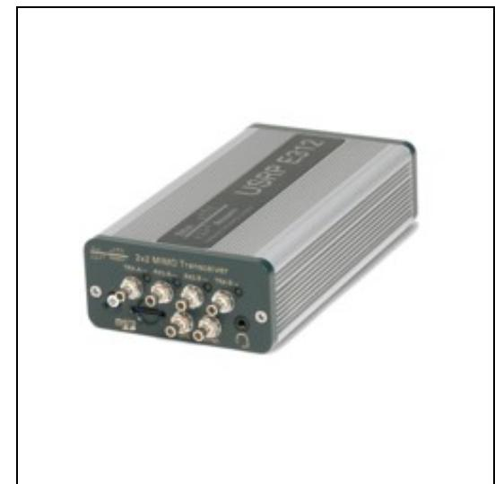
The USRP E310 MIMO XCSR daughterboard features an integrated MIMO capable RF frontend.
