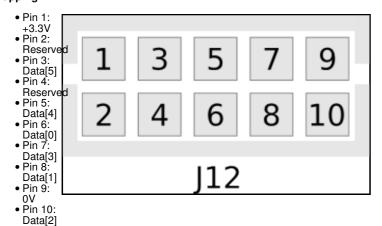
The hardware power on state and UHD initial state for the front-panel GPIOs is high-Z. For the E3xx, there are no external pull-ups/pull-downs for the GPIO pins, but the FPGAs do have them and they are configured as follows: E3xx: pull-down.
