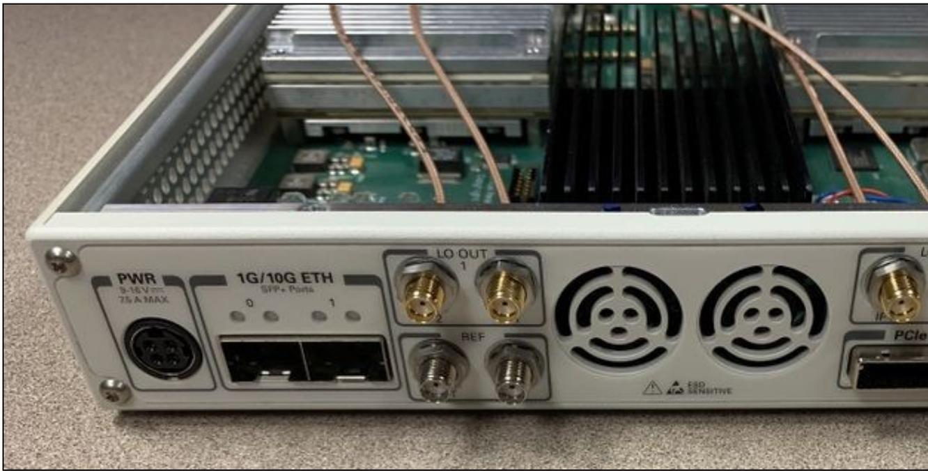
*X310 Back Plate With SMA to MMCX Cables*
