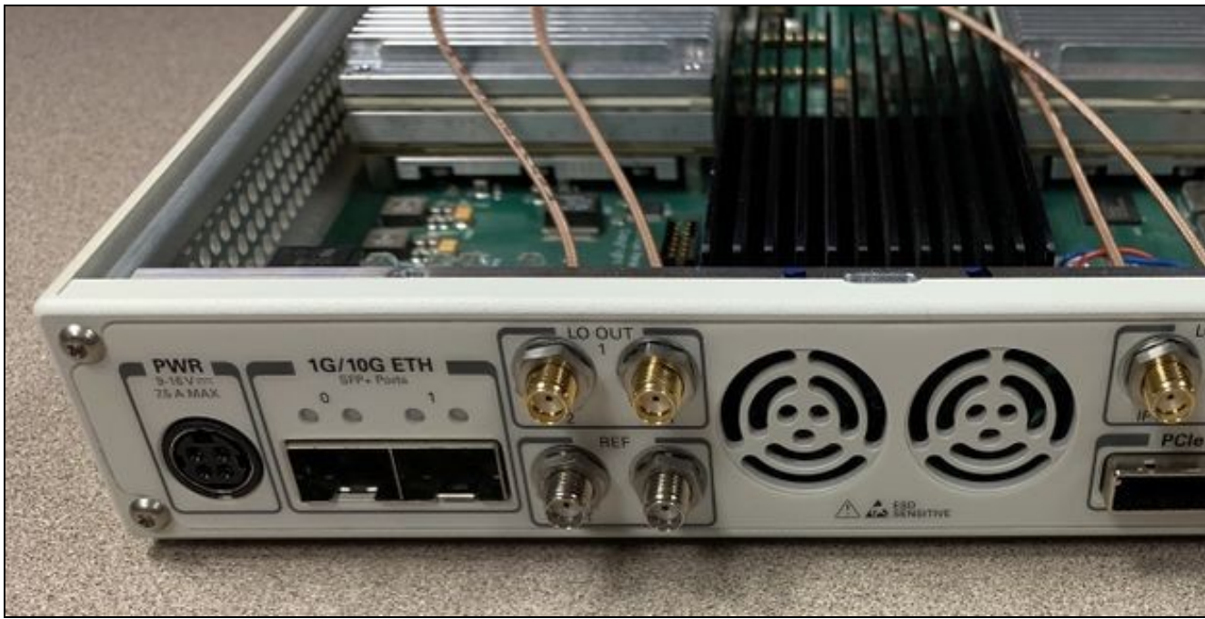
X310 Back Plate With SMA to MMCX Cables
