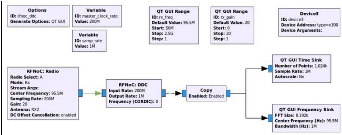
The USRP Source and Sink blocks use the `multi_usrp` API, whereas the RFNoC:Radio block uses the RFNoC API. In general, unless RFNoC features are desired, there is no need to use the RFNoC:Radio block. The RFNoC:Radio block is most useful when its output is connected directly to another RFNoC block. Below is a list of differences as well as a GRC screenshot to help differentiate between the two blocks.
