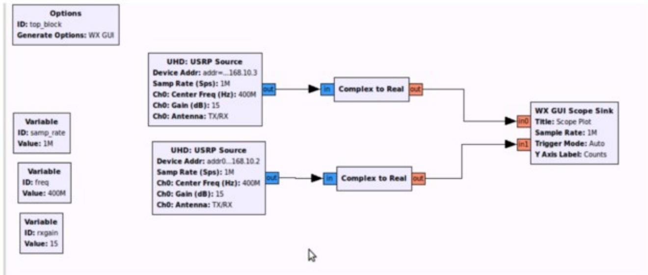
Figure 3– GRC – Un-Synchronized Reception with Two USRP N200/210s
