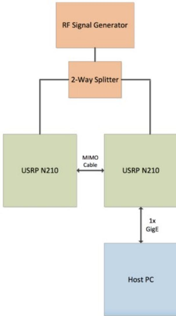
Figure 5 – N200/N210 2x2 Reference Design and Test
