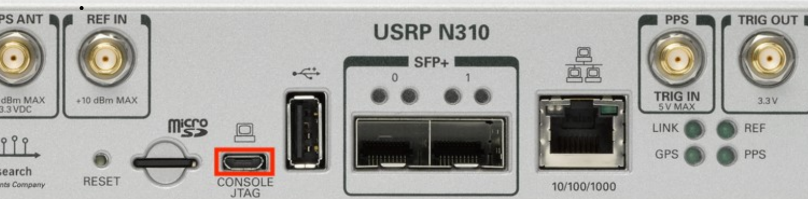
Figure 1: N310 Rear Panel with serial port emphasized.
