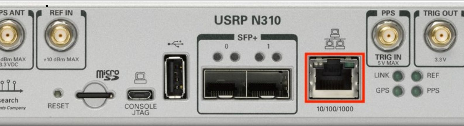
Figure 1: N310 Rear Panel with MGMT port emphasized.
