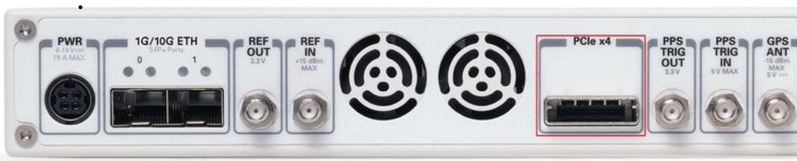
Figure 5: X310 Rear Panel with PCIe port emphasized.
