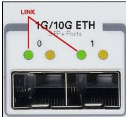
Figure 2: X310 SFP+ ports with link and data LEDs.
