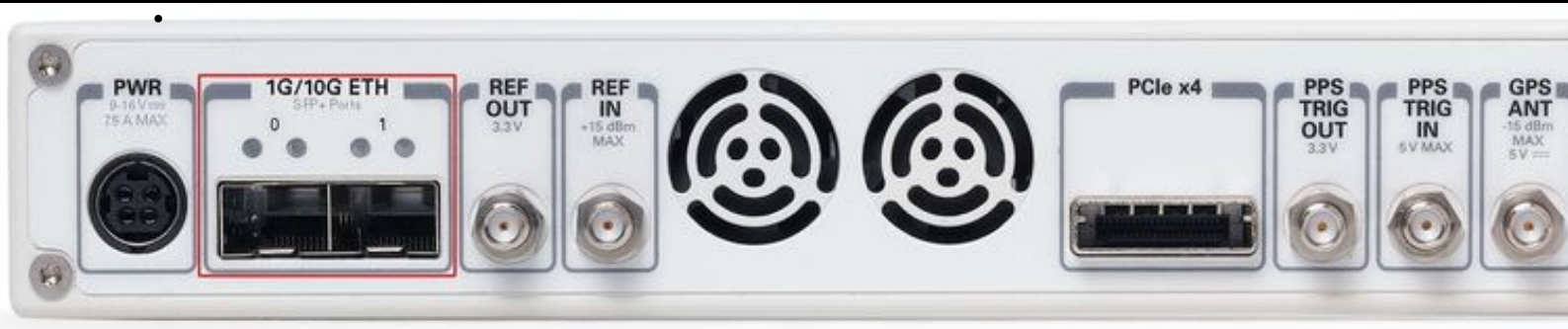
Figure 1: X310 Rear Panel with SFP+ ports emphasized.
