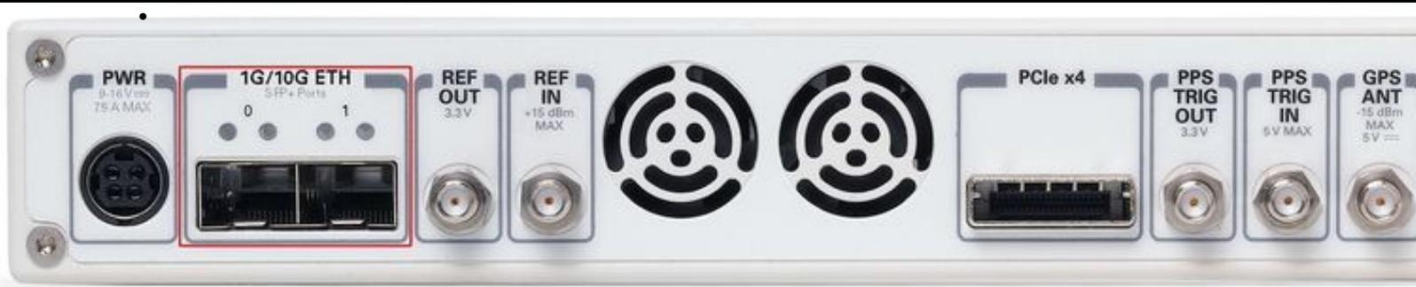
Figure 1: X310 Rear Panel with SFP+ ports emphasized.
