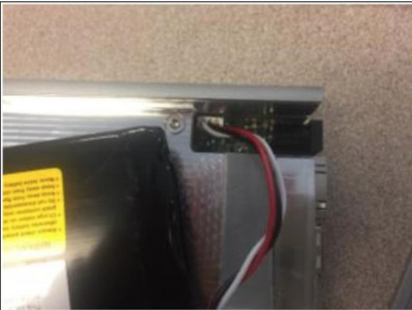
7. Place the replacement cell in the battery tray. Make sure the battery wires will not impinge on the top cover of the USRP E312.
