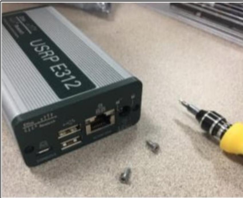
2. Carefully pry off the rear panel and slide off the top cover of the USRP E312.
