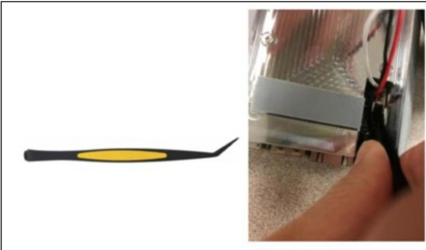
5. Gently extract the connector from connector J1 on the E312 motherboard.
