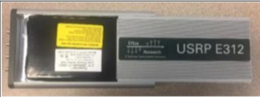
9. Replace the rear panel. Tap on the edges to ensure it is flush with the enclosure.
