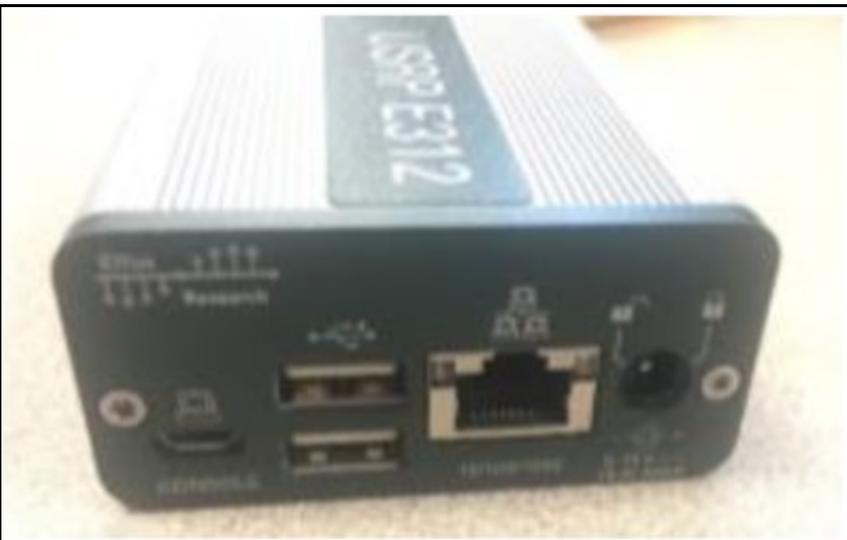
11. Plug in the USRP E312 unit to charge the battery. The battery should be fully charged within 2 hours. Do not charge the battery for more than 24 hours. Once the battery is charged, the USRP E312 unit can be unplugged, powered on, and operated standalone.
