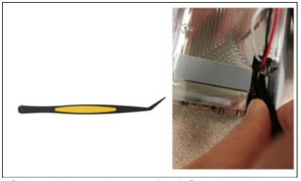
5. Gently extract the connector from connector J1 on the E312 motherboard.
