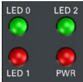
**Power LED** The USRP X4x0's PWR LED is reserved to visually indicate the user the device's power state. Power LED Behavior describes what each LED state represents.
