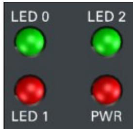
**Power LED** The USRP X4x0's PWR LED is reserved to visually indicate the user the device's power state. Power LED Behavior describes what each LED state represents.
