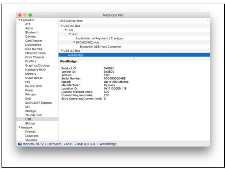
Once the USRP firmware is loaded -- more on this in the next section -- the device with "morph" on the bus, which will change the device name and capabilities. The following screenshot shows the hardware information of a USRP B210 after the firmware was successfully loaded.
