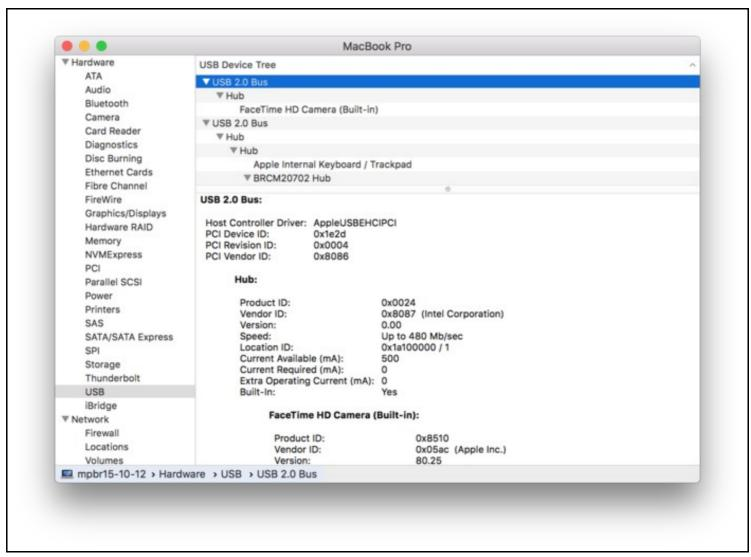
In the upper pane, scroll down until you find an entry for either <code>Westbridge</code> or <code>USRP B2\*</code>. The following screenshot shows the hardware information of a USRP B210 immediately after it is plugged in and powered up.
