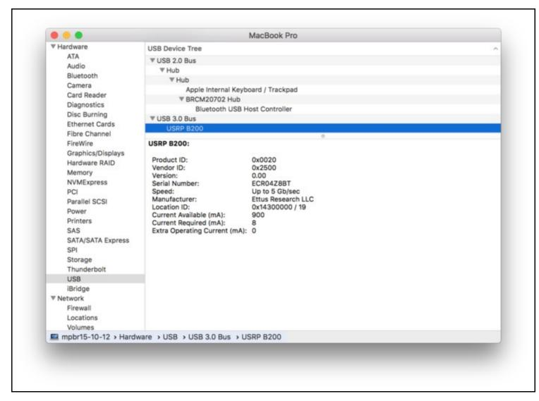
When a USRP B-series device is plugged into a USB port and powers up, both the firmware and FPGA images need to be loaded for it to work with UHD. These binaries will be loaded when UHD is started and pointed to the B-series USRP, regardless of the application, host computer, or OS.
