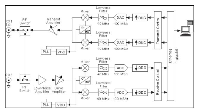
The analog bandwidth is the amount of useful bandwidth (3 dB) between the RF port and IF/baseband interface of an RF channel. Typically this bandwidth is set by IF or baseband filters on the daughterboard, which are designed to avoid aliasing when paired with a USRP motherboard with given ADC/DAC sample rates.
