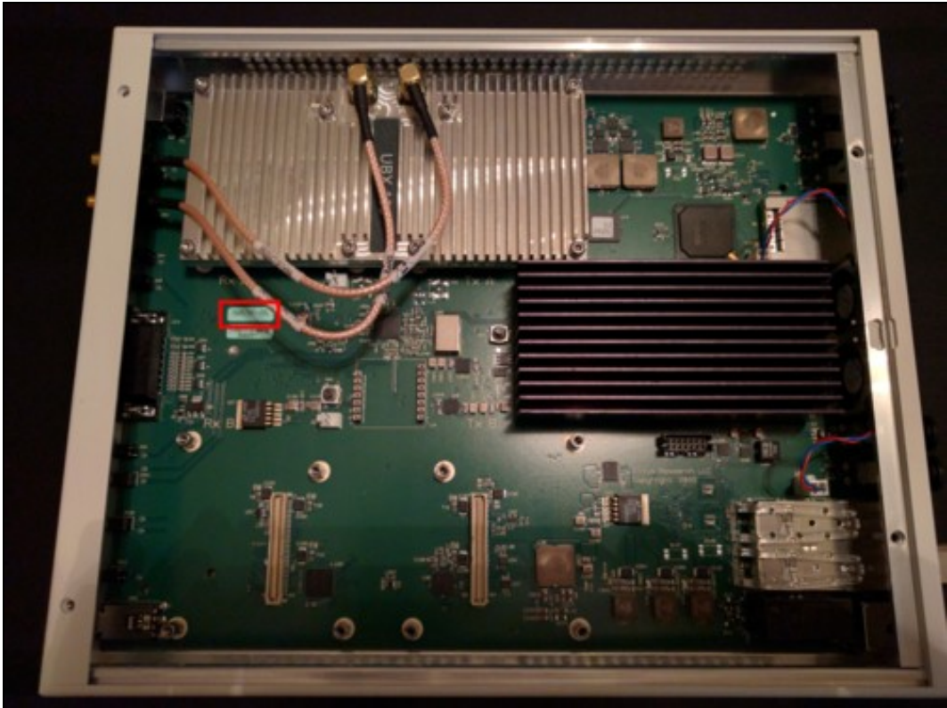
The USRP X300/310 motherboard has a sticker that identifies the product and revision. The sticker is outlined in red.
