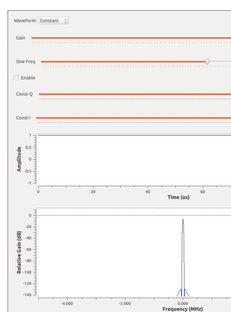
Signal type: Sinusoid || Gain: 1: Now the wave type is set to 1, being the next option available. The gain is unchanged to show how it holds the same value in the readback register.
