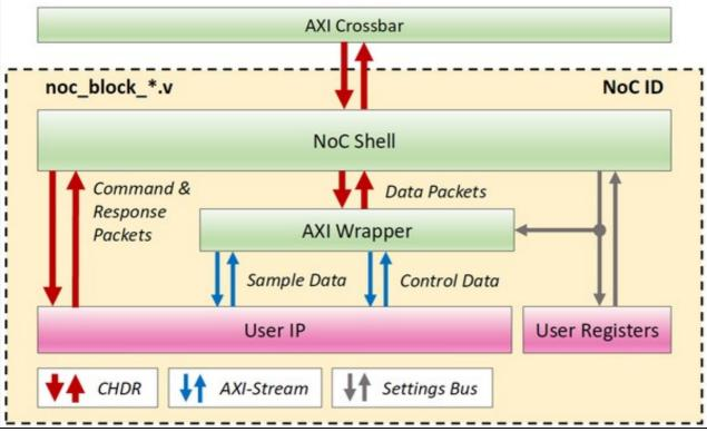
From NoC Shell: At the top of the figure you can see the AXI Crossbar, were all the computation engines are wired up together. This is not part of our UUT in particular. However, the connection between the crossbar and our UUT - NoC Shell can be tested within our code. From here we are taking the set\_data/addr/stb, which are readback registers and provide information from this interface.
