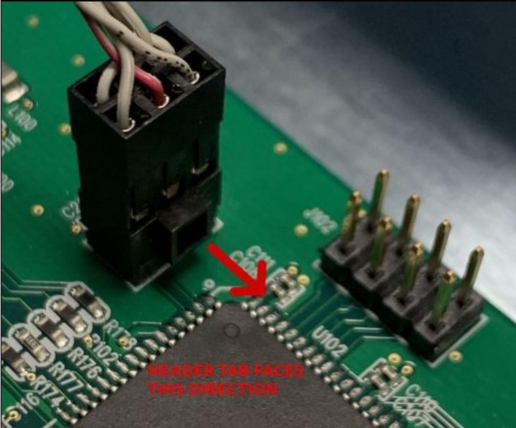
Note: If you plug the header in backwards, `avrdude` is expected to return a `please check your connections` message after a programming failure. See the section "Troubleshooting" at the bottom of this document for more detail.
