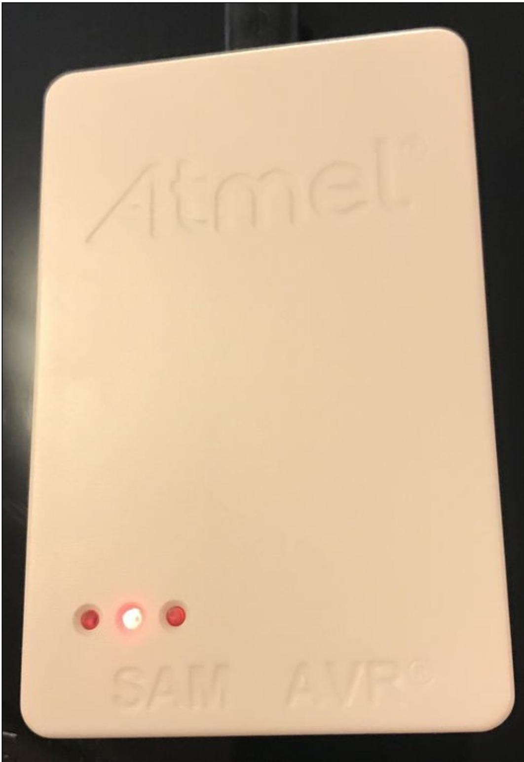
Supply power to the Octoclock with the 6V power brick. You should see the Octoclock's Power LED come on and the left LED (green) on the ATMEL-ICE programmer illuminate, such that the left 2 LEDs are lit. The overall setup should look something like this:
