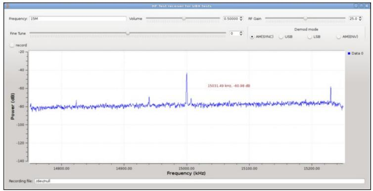
The 15MHz WWV carrier is received at approximately 40dB above the notional noise floor, with easily understood audio.
