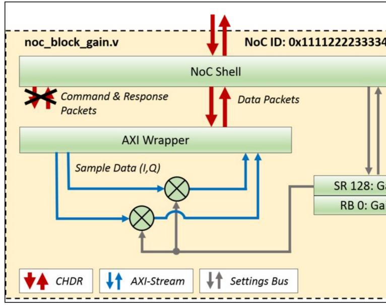
Open the file rfnoc-tutorial/rfnoc/fpga-src/noc\_block\_gain.v that contains the RFNoC block skeleton code that was created when the \$ rfnocmodtool add gain command was run and modify the following (BOLD indicates changes to the skeleton code).
