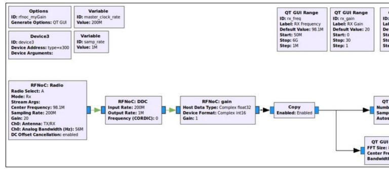
NOTE: Copy Block: In the RFNoC domain, streams of data can not be split as easily as they are in the GNU Radio domain. The ?copy? block depicted in the screenshot above serves the function as a stream splitter . It?s main purpose, when ?enabled?, is to copy the samples it is getting at its input and putting then into the output, but here it is also serving as a boundary between a RFNoC-domain and a GNURadio-domain. In the flowgraph above. after
