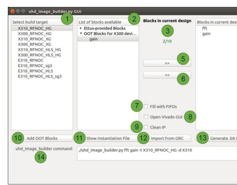
1. Select build target: In this panel the available build targets are listed. This list may vary depending on which branch of the FPGA repository this user is using. Only RFNoC targets are listed. The build type descriptions are:
