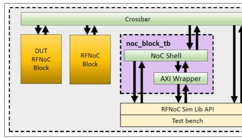
**NOTE:** The noc\_block\_tb block is an instantiation of the noc\_block\_export\_io that is used in testbenches to communicate to the RFNoC architecture. This makes it possible to talk ?RFNoC? to the user?s custom block and as such the custom block has a complete RFNoC experience (signaling, flowcontrol, addressing, etc)
