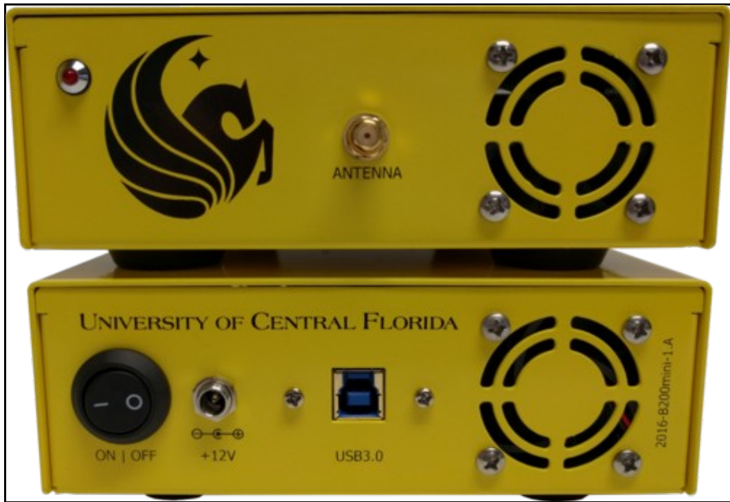
Figure 8: Photograph of the front of the USRP enclosure. A single antenna is switched rapidly between the transmit (TRX) and receive (RX2) ports. The rear panel has ports for power and data (USB3.0). The dimensions of the system are 18x15x5cm (7x6x2in.) and has a mass of approximately 630g (1.4lbs.).
