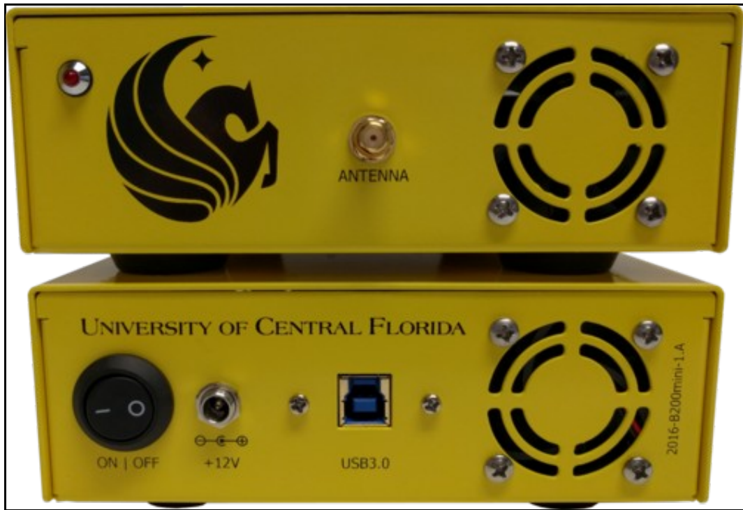
Figure 8: Photograph of the front of the USRP enclosure. A single antenna is switched rapidly between the transmit (TRX) and receive (RX2) ports. The rear panel has ports for power and data (USB3.0). The dimensions of the system are 18x15x5cm (7x6x2in.) and has a mass of approximately 630g (1.4lbs.).
