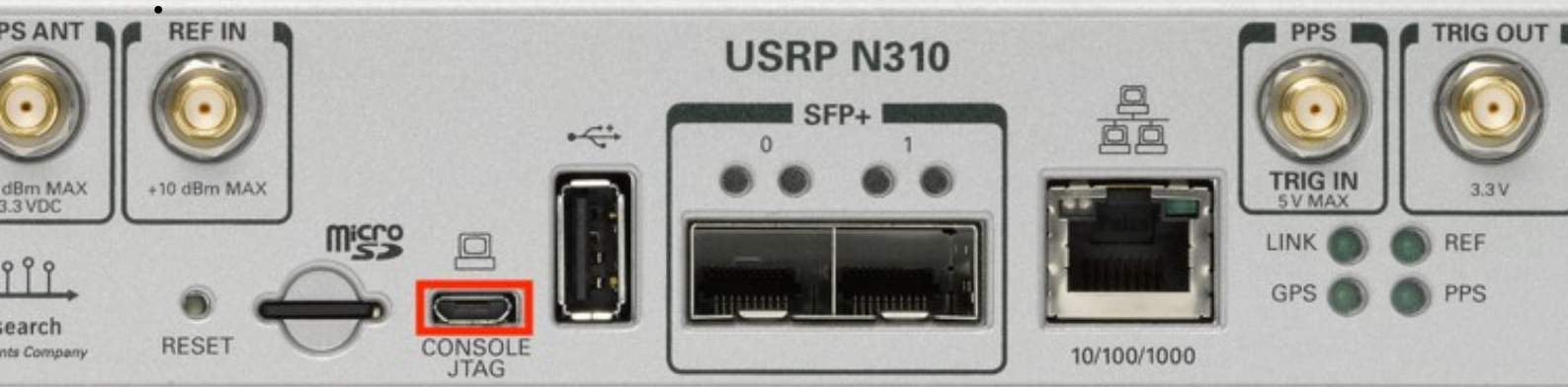
Figure 1: N310 Rear Panel with serial port emphasized.
