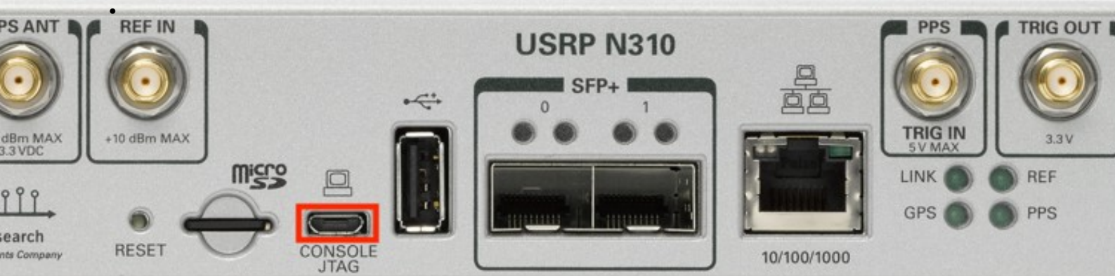
Figure 1: N310 Rear Panel with serial port emphasized.
