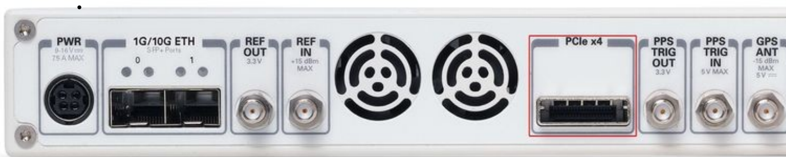
Figure 5: X310 Rear Panel with PCIe port emphasized.
