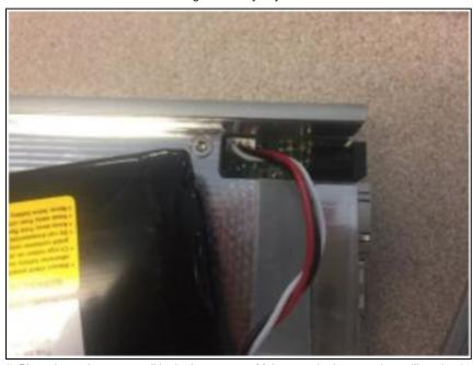
7. Place the replacement cell in the battery tray. Make sure the battery wires will not impinge on the top cover of the USRP E312.
