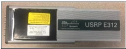
9. Replace the rear panel. Tap on the edges to ensure it is flush with the enclosure.
