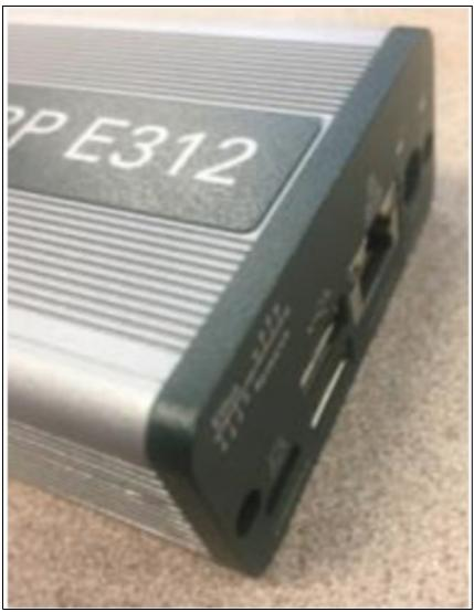
10. Replace the rear panel two retaining screws with a Torx T8 driver.
