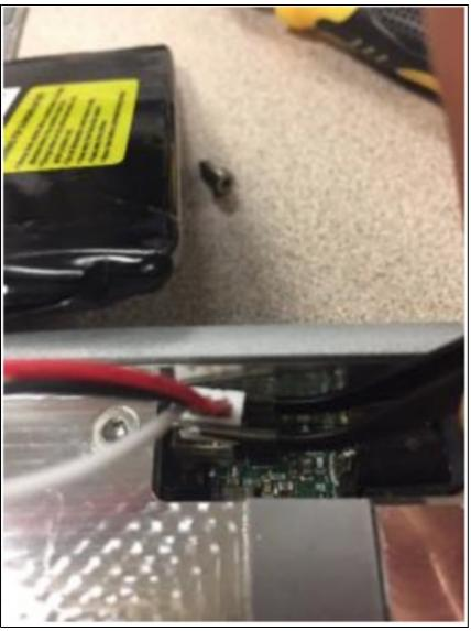
6. Insert the white plastic connector of the replacement USRP E312 battery cell into connector J1 on the motherboard. Ensure that the white wire is closest to the T8 Torx screw securing the battery tray to the USRP E312 motherboard.
