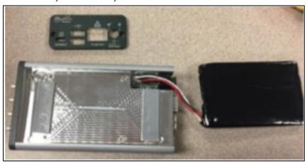
4. Grasp the sides of the white plastic battery cell connector with a pair of bent-tip tweezers.
