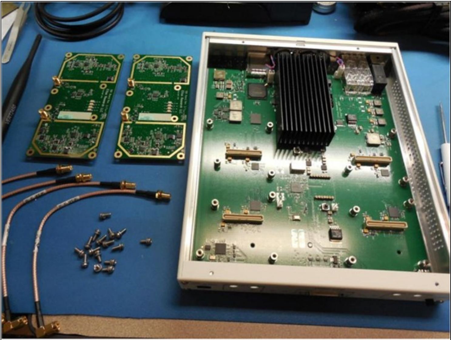
Line up the 8 screw holes on the Daughterboard with the USRP Motherboard standoffs (they only go one way).
