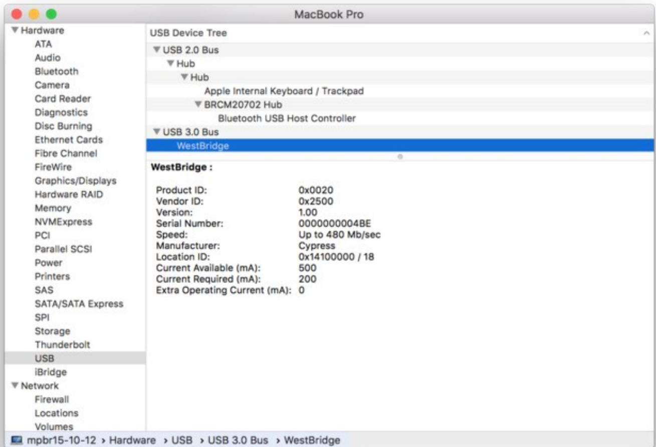
Once the USRP firmware is loaded -- more on this in the next section -- the device with "morph" on the bus, which will change the device name and capabilities. The following screenshot shows the hardware information of a USRP B210 after the firmware was successfully loaded.
