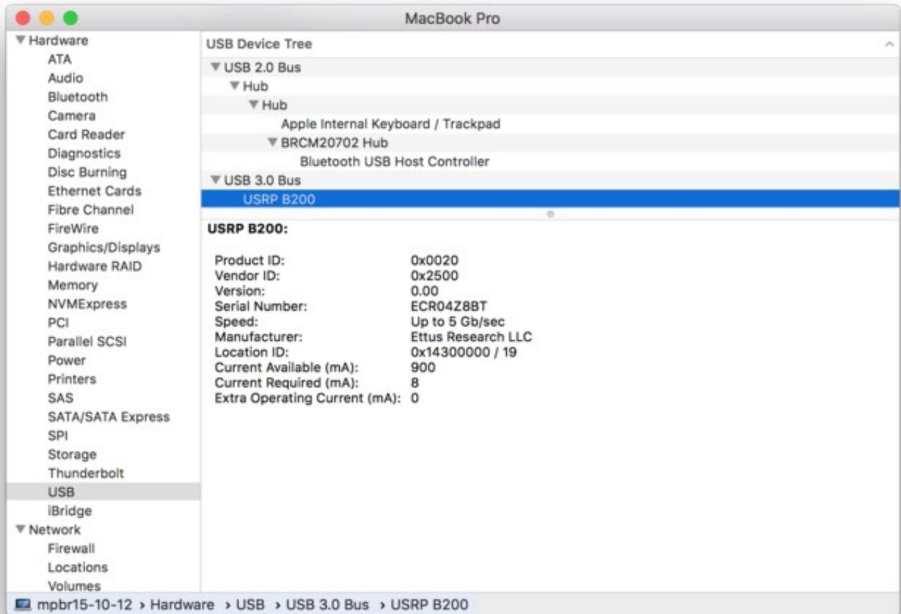
When a USRP B-series device is plugged into a USB port and powers up, both the firmware and FPGA images need to be loaded for it to work with UHD. These binaries will be loaded when UHD is started and pointed to the B-series USRP, regardless of the application, host computer, or OS.
