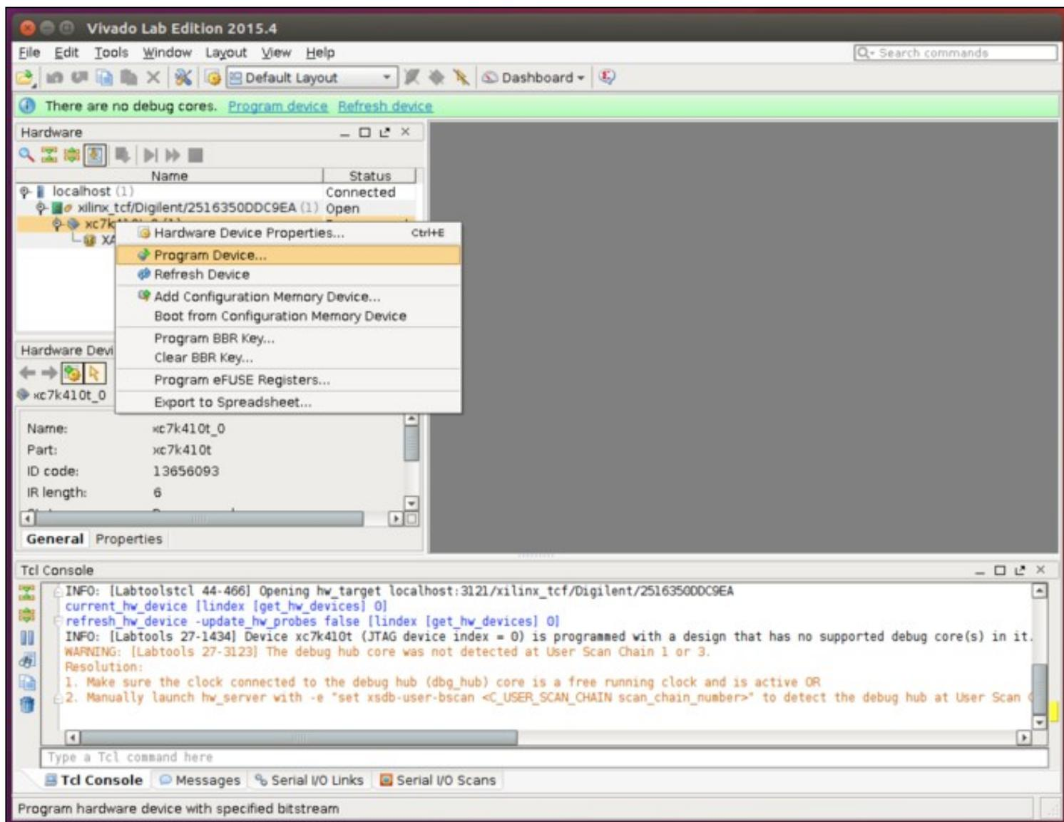
This will popup a new window. Click on the file selection button and navigate to the location of the UHD FPGA images, and select the correct FPGA image for your device. (/usr/local/share/uhd/images)
